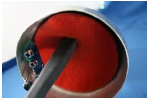
Picture G – Padding that completely covers the wires
