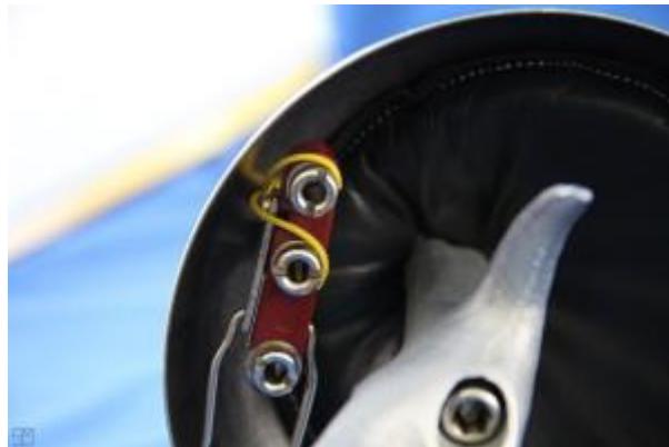
Picture B – Wires incorrectly wrap around posts
