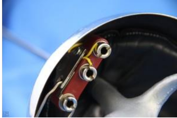
Picture C – Inability to inspect the length of the wires
